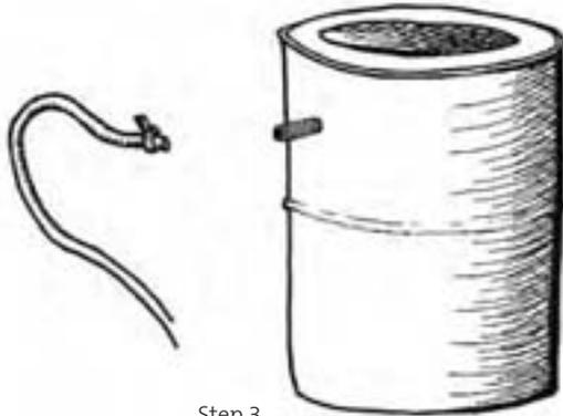
B) Screw the gray 1 1/4" barbed fitting onto the threads of the white male coupling.
