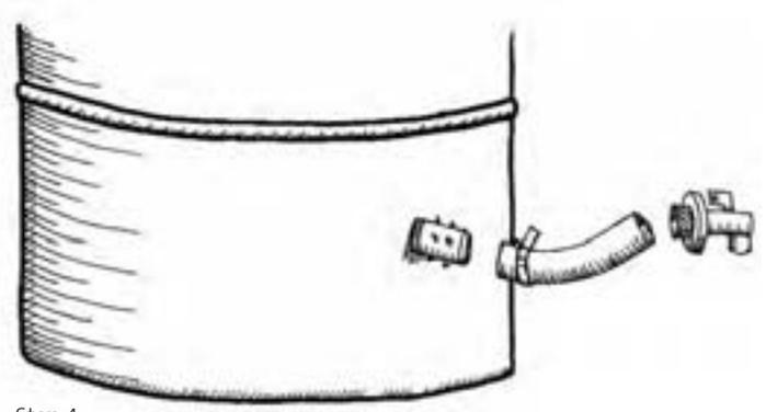
B) Put the small hose clamp onto one end of the 5-inch section of garden hose. Push the hose onto the barbed fitting and tighten the clamp.
